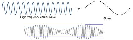
Amplitude modulated carrier wave
